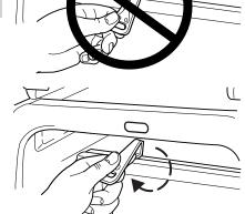
7. Tighten the child safety seat tether strap according to the manufacturer's instructions.
